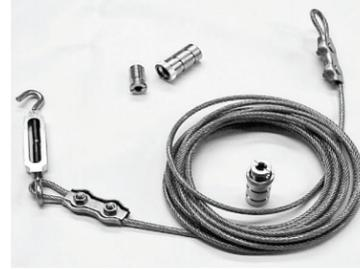
This hardware can be used with spring clips to draw a portion of a safety cover securely around the perimeter of a fixed pool feature. It can also be used in association with expansion anchors, threaded eye bolts and spring clips to create a safe attachment to an object into which expansion anchors can be permanently set.
